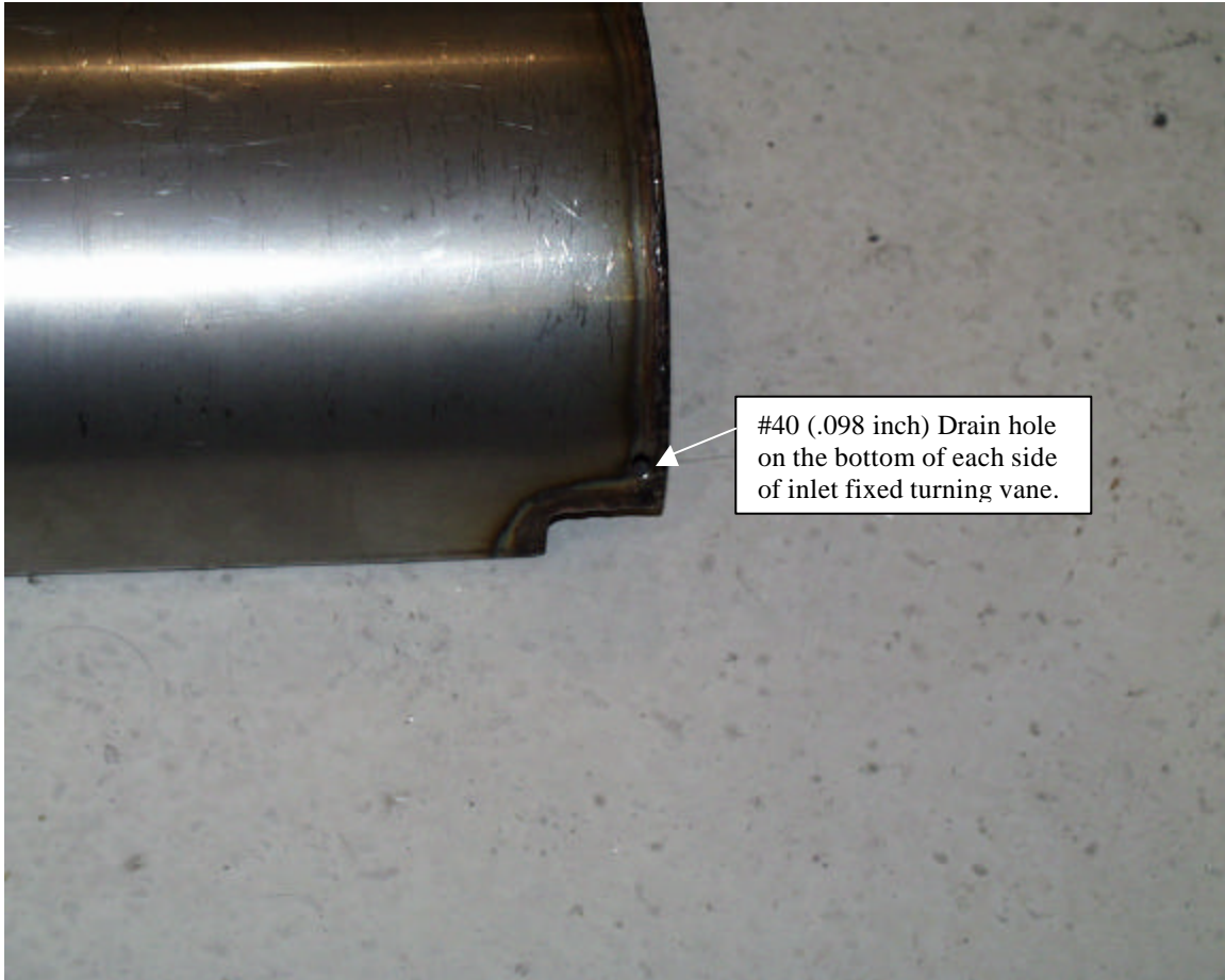
Figure 2. Location of Fixed Turning Vane Drain Holes
